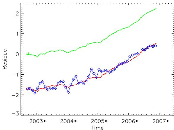
Figure 5. Residue as a function of time. The figure is similar to Fig. 3, and the legend of that figure also applies to this one. The green curve represents  $\Delta r$ , the calculated increase in the residue from degradation of the reflectance alone. The red curve is basically the green curve but then shifted vertically to the value of the global monthly mean residue at the first available data point.
