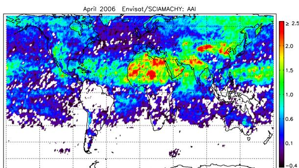
Figure 2. Global map of the monthly mean SCIAMACHY AAI for April 2006. Compared to Fig. 1, the AAI shows anomalously high values. This is caused by degradation of the optics of the SCIAMACHY instrument.
