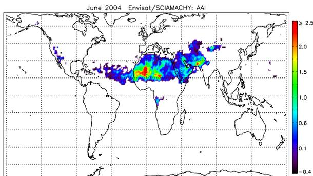
Figure 1. Global map of the monthly mean SCIAMACHY AAI for June 2004. The ‘Global Dust Belt’ is clearly visible, illustrating the transport of desert dust over the North Atlantic ocean.
